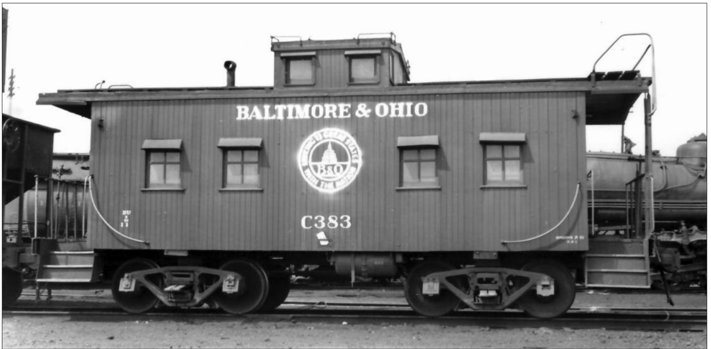
B&O C-383 - was last repainted at B&O's Du Bois, Pennsylvania, shops in August of 1953. This car exhibits upgraded trucks, and side grab irons and ladder roof handholds have been added, although it still retains its coach-type steps.
